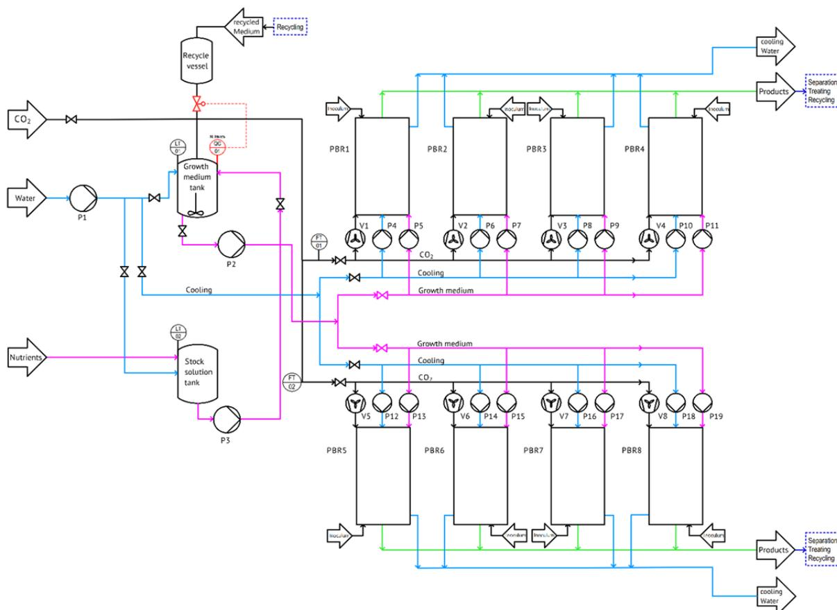
Figure 3: Process flow scheme of the cultivation module
